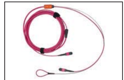
FM4MMB1010M, FX MPO Trunk, OM4, MPO-12 (Male to Male), Type-B, 1 x MPO-12 (12 fibers), 10 m, OFNP, Mini-Distribution 4.8 mm (Double-Jacket), Erika Violet Jacket
